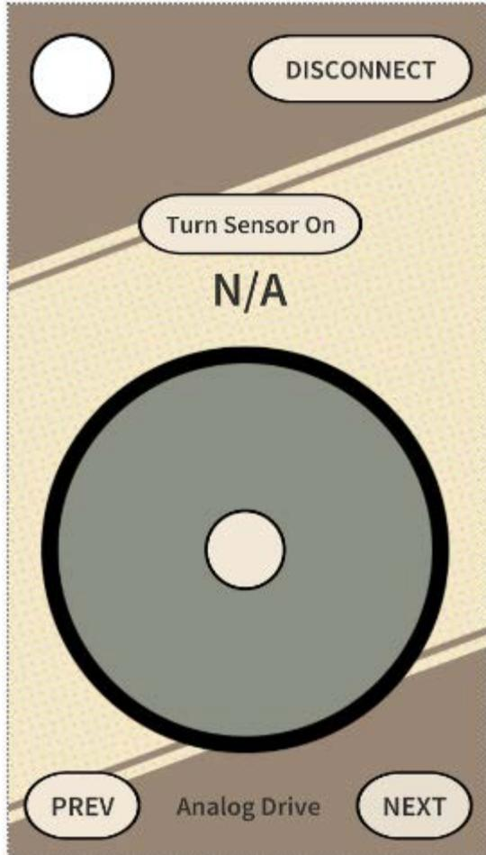
The Analog Drive gives you a better feel to control the robot. You can Turn Sensor On and get distance readings from the sonar sensor. Try the NEXT screen for voice control.
