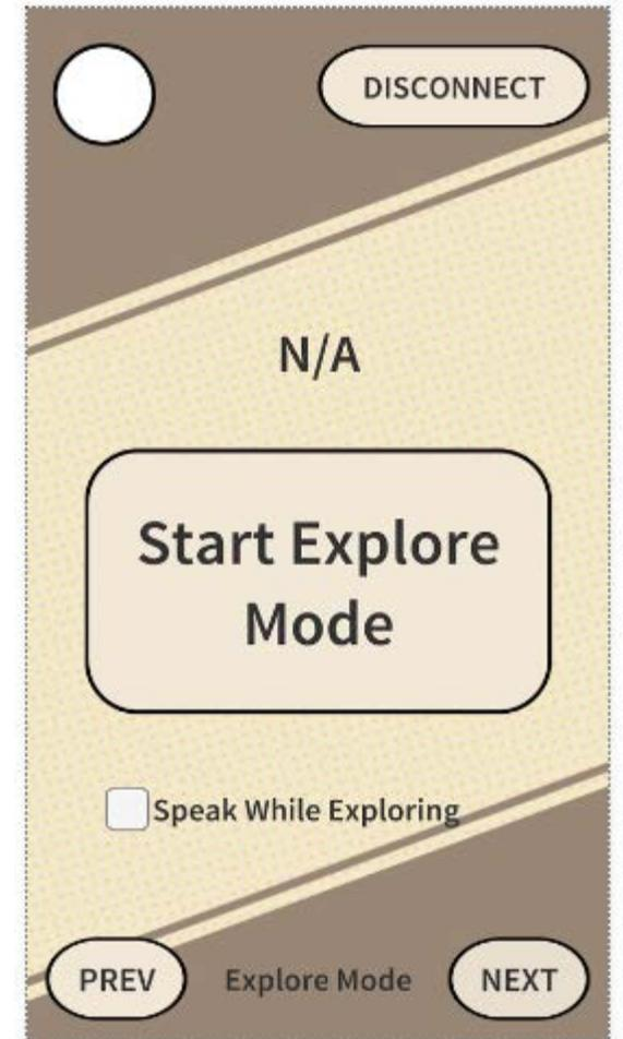
Explore mode uses the sonar sensor and can speak while exploring
